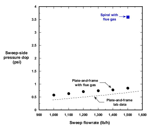
Field data from NCCC is consistent with lab results, and confirms much lower air sweep pressure drop in plateand-frame modules
