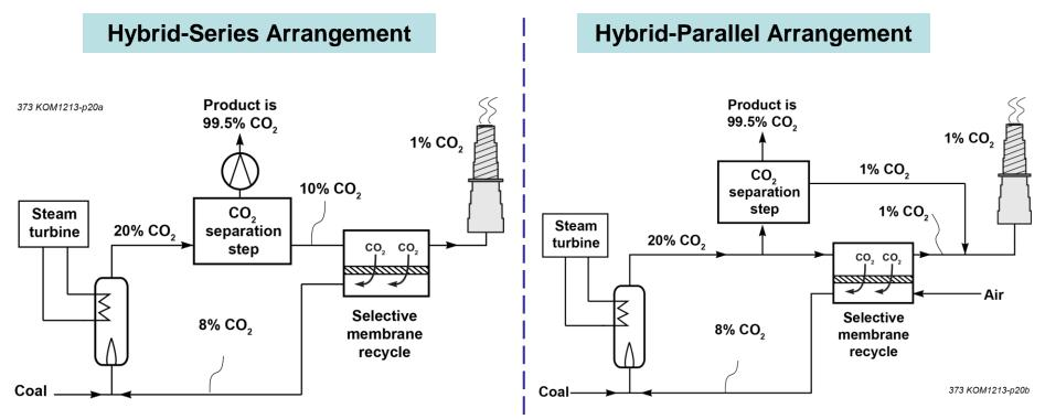
Depending on the arrangement, the selective recycle membrane can:
